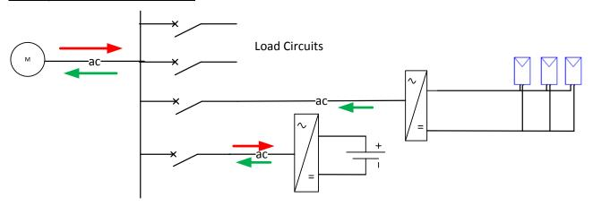
Installed Capacity = solar inverter rating + battery inverter rating Not export limited.
