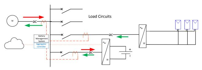
Installed Capacity = solar inverter rating + battery inverter rating
