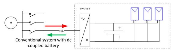
Figure 2 Example of a DC coupled solar and battery storage system
