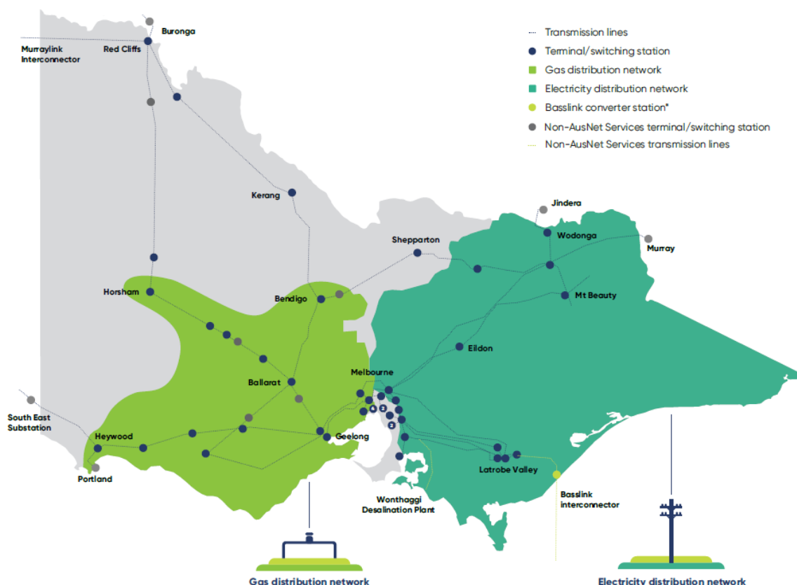
Figure 1.1: AusNet's Electricity and Gas regions
