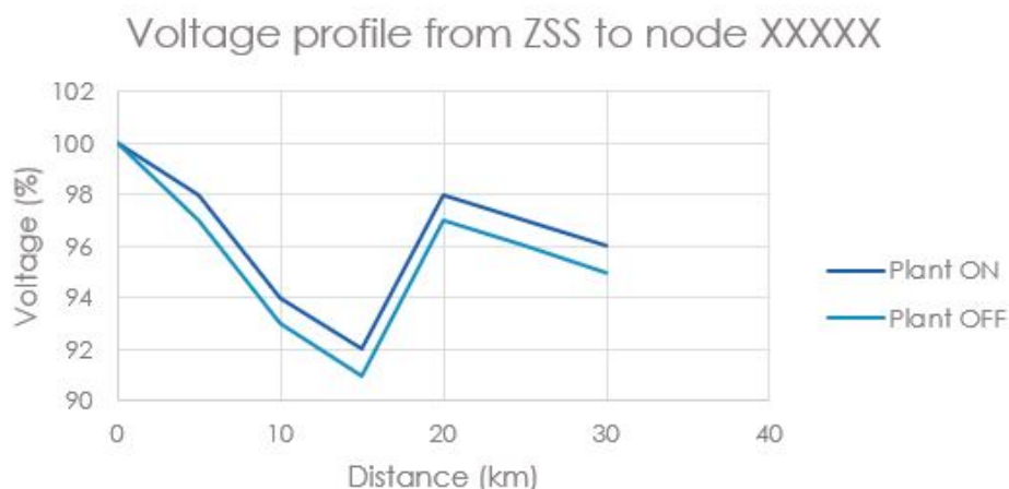
Figure 2 Voltage profile needs to be illustrated for different network configurations in maximum and minimum load conditions
